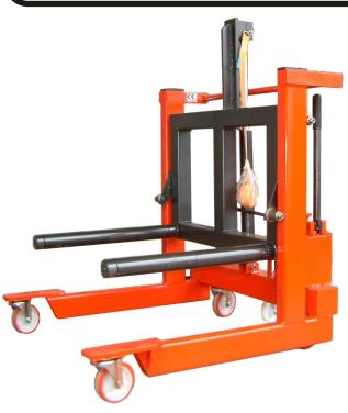
The C.A.M. Commercial Wheel Removal Trolley enables wheel assemblies of up to 1000 Kg (approx. 2200 lbs), to be removed and re-assembled to vehicles by just one man.
